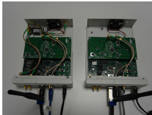
Figure 3.12: N210 Ettus devices with the XCVR2450 daughterboard installed. A two-antenna cognitive receiver is composed of two N210 boards connected through a MIMO cable.
