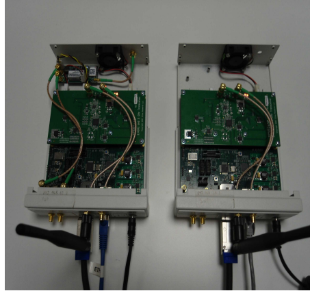
Figure 4.2: N210 Ettus devices with the XCVR2450 daughterboard installed. A two-antenna cognitive receiver is composed of two N210 boards connected through a MIMO cable.
