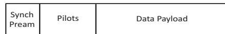
Figure 2.7: A data packet composed of a header (a synchronization preamble and pilots) and the data.
