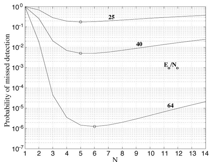
Fig. 3. Probability of missed detection as a function of the number of subintervals ( $P_{FA} = 10^{-5}$ ,  $\Delta fT_o = 1$ ).
