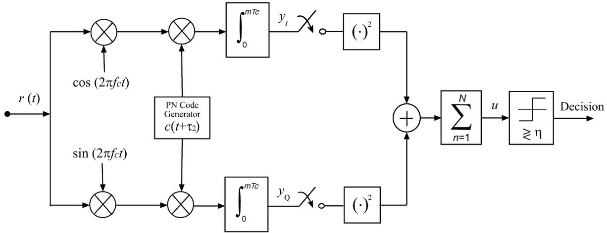
Fig. 1. Noncoherent receiver block diagram.
