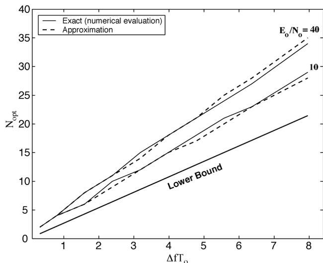
Fig. 2. Optimum number of subintervals as a function of  $\Delta fT_o$  ( $P_{FA} = 10^{-5}$ ).
