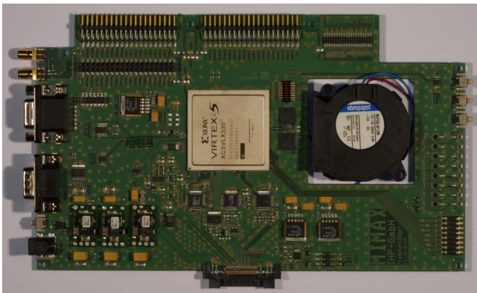
Figure 6. MIMAX baseband printed-circuit-board
