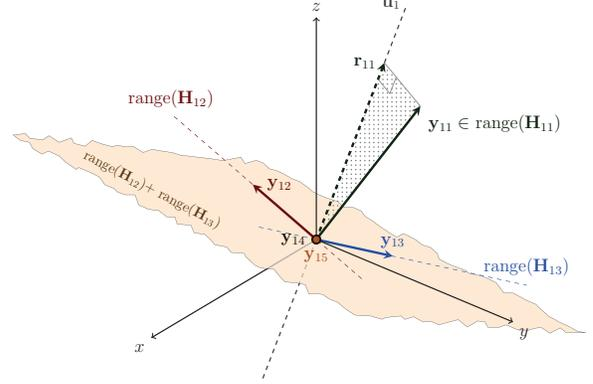
**Fig. 1.** Signal space at the receiver of user 1 for the  $(3 \times 3, 1)^5$  scenario with rank-one MIMO channels. In this case, user 1 only sees the interference coming from users 2 and 3 (users 4 and 5 employ ZF-BF), which spans a subspace of dimension 2. The direction orthogonal to that subspace provides the required signalling dimension free of interference ( $\mathbf{u}_1$ ).
