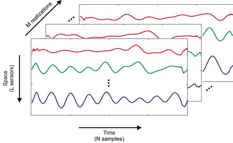
Fig. 1. Observations consist of  $M$  space–time snapshots of dimensions  $L \times N$ , each one representing the signals acquired by  $M$  sensors during  $N$  time instants.
