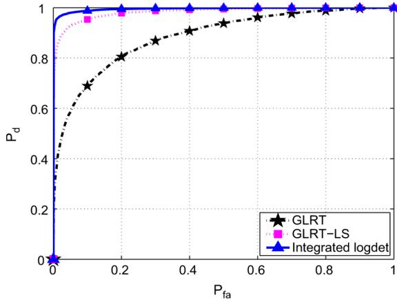
Fig. 2. ROC for  $L = 3$ ,  $\text{SNR} = -5$  dB,  $N = 48$ ,  $M = 150$ ,  $\alpha = 0.9$ ,  $\nu = 10/N$ .
