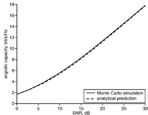
**Fig. 1** Comparison between theoretical ergodic capacity and analytical prediction of (4) for uncorrelated Rayleigh channel against SNR
