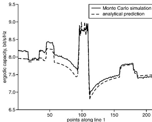
**Fig. 3** Simulated ergodic capacity along line 1 of Fig. 2 for  $SNR = 15$  dB
