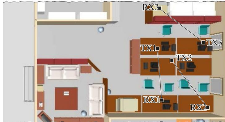
**Fig. 5** Plan of the measured scenario. The distances between users 1, 2, and 3 are approximately 3, 3.4, and 3.2 m, respectively. Notice that the line-of-sight of the link between TX3 and RX3 is blocked by shelves
