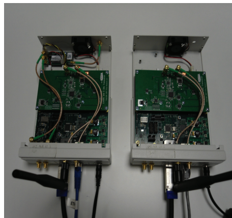
Fig. 2. N210 Ettus devices with the XCVR2450 daughterboard installed. A two-antenna cognitive receiver is composed of two N210 boards connected through a MIMO cable.
