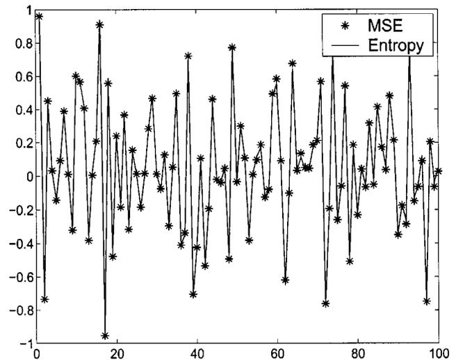
Fig. 2. Error sequence at the output of an LTE for the MSE solution ("\*"), and the minimum entropy solution (solid line). Channel  $H(z) = 0.87 + 0.44z^{-1} + 0.23z^{-2}$ ,  $m = 7$ ,  $d = 3$ , SNR = 10 dB, kernel size  $\sigma^2 = 1$ , and 100 training samples (batch training).
