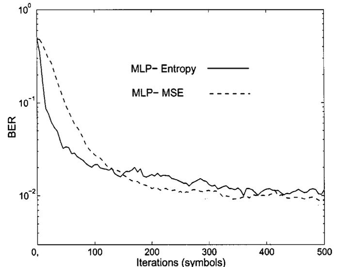
Fig. 6. Convergence of the BER with the number of iterations for the MSE (dashed line) and the minimum entropy (solid line).
