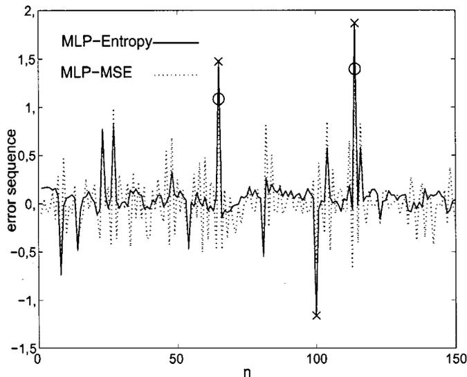
Fig. 7. Error sequence at the output of nonlinear equalizer for the MSE solution (dashed line), and the minimum entropy solution (solid line). Circles and crosses indicate classification errors for MSE and entropy, respectively.
