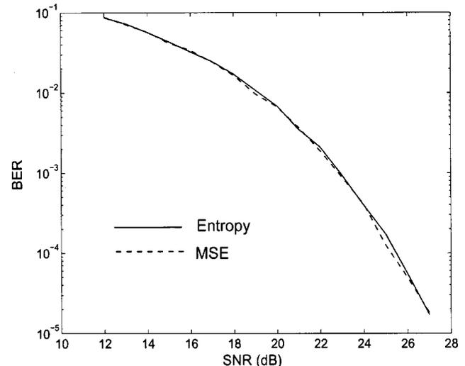
Fig. 3. BER comparison for the minimum entropy (solid) and MSE (dashed) linear equalizers. Channel  $H(z) = 0.35 + 0.8z^{-1} + z^{-2} + 0.8z^{-3}$ ,  $m = 9$ ,  $d = 5$  and 100 training samples (batch training).
