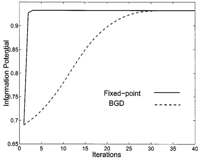
Fig. 1. Information potential  $V(e)$  versus iterations for the fixed-point and the batch gradient descent (BGD) algorithms.
