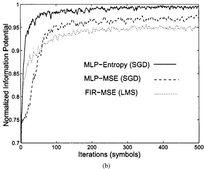
Fig. 4. Convergence characteristics of online adaptive algorithms for a linear equalizer with  $m = 7$  coefficients (dotted line) and an MLP(7-4-1) trained with MSE (dashed line) and minimum entropy criteria (solid line) using a window size of  $N_w = 5$  samples. (a) MSE. (b) Normalized information potential.
