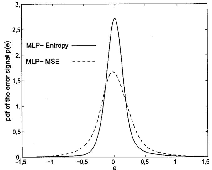
Fig. 5. Estimated pdf of the error at the equalizer's output for the MSE (dashed line) and the minimum entropy (solid line).
