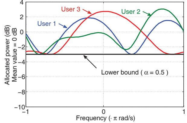
**Fig. 2.** Power allocation over frequency for each of the three users. Results after algorithm convergence at iteration 500 with  $L = 5$  and  $\alpha = 0.5$ .
