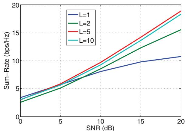
Fig. 5. Sum-Rate performance for  $\alpha = 0.5$  and different orders,  $L$ , of the space-time precoders and decoders.
