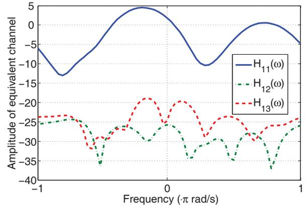
**Fig. 3.** SISO equivalent channels for the receiver 1: the direct channel (solid line) and two interfering channels (dashed line).
