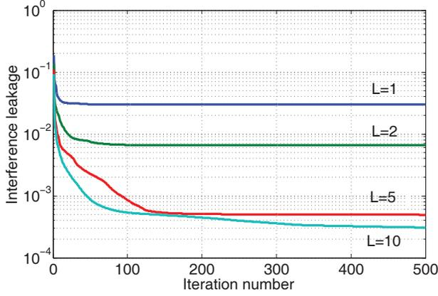
**Fig. 1.** IL vs. number of iterations for different orders,  $L$ , of the space-time precoders and decoders and parameter  $\alpha = 0.5$ .
