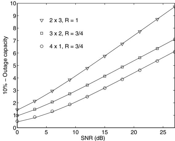
Fig. 1. 10%-Outage capacity of OSFBC for different MIMO configurations as a function of the average SNR at the receiver antennas. The curves compare the analytical predictions of (17) (solid lines) with Monte Carlo simulations (markers).
