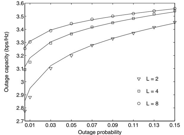
Fig. 2. Outage capacity of  $3 \times 3$  OSFBC, as a function of the outage probability, for different channel lengths.
