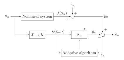
Figure 1: Kernel-based adaptive system identification. Figure adapted from [8].
